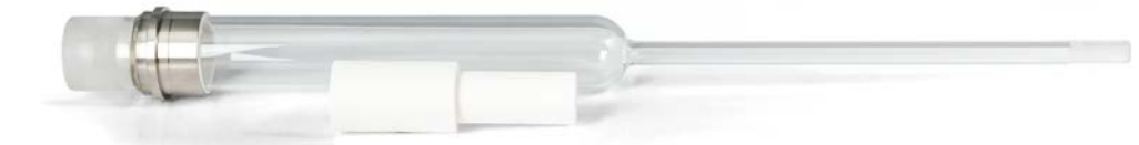
Protective tube made of fused silica (order no. 6.219.1-71.2.00)
