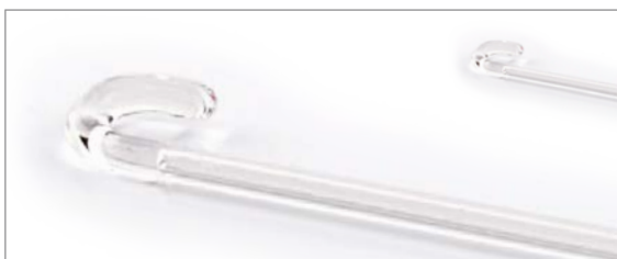
Fused silica pushrod for expansion, spherical type (order no. TMA40200A05.023)
