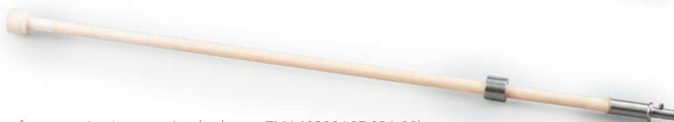
Alumina pushrod with pushrod cap for expansion/penetration (order no. TMA40200A07.021-00)
