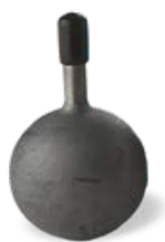
2 Spherical vessel, titanium, 8.6 ml, 10.0 g
