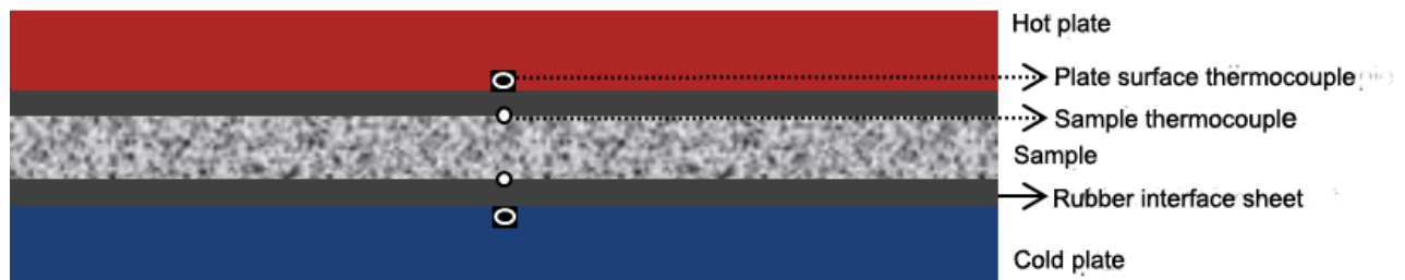
3 HFM and GHP arrangement for sample surface thermocouples
