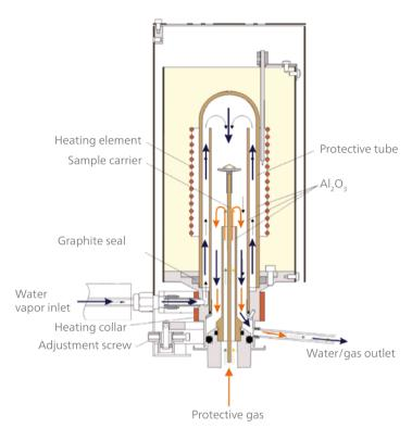
Cross-section of the water vapor furnace
