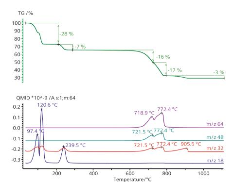
Thermogram of blue vitriol in combination with the ion current curves of m/z 18, 32, 48 and 64
