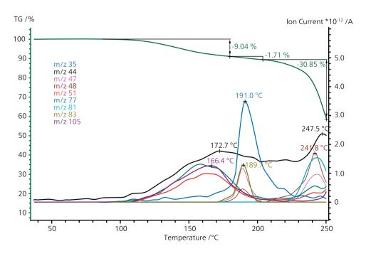
Correlation of the mass loss steps and the detected gases. m/z 35 can most likely assigned to HCl.
