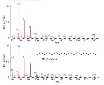
Comparison of the mass spectrum, measured at 270°C (top picture) with the spectrum of the NIST-MS library (picture below)
