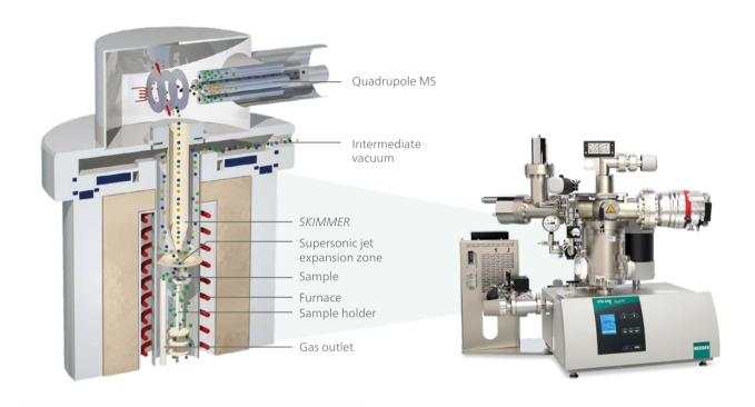
Shortest possible coupling solution via special supersonic jet gas transfer
