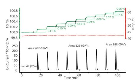
Isothermal treatment of CaO (177.8 mg) on a Pt grid sample carrier at 43°C in a dry argon atmosphere with pulses of 250  $\mu$ l of CO  $_2$
