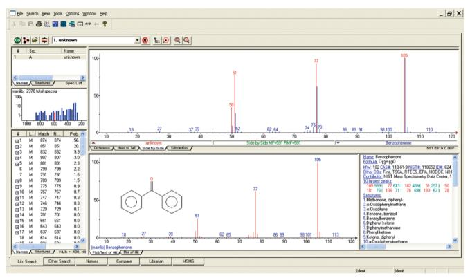
Direct export of the MS results at 166°C into the NIST database for identification of the evolved gases
