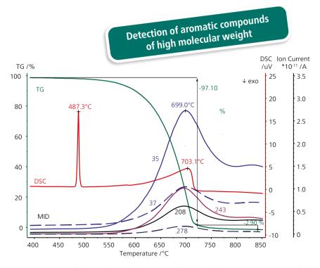
Comparison of the mass loss and DSC curve of  $\mbox{PbCl}_2$  with the ion current curves of the fragment ions
