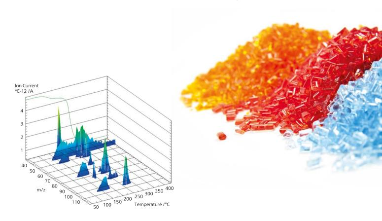
3-D plot of a TGA-MS measurement on an unknown polymer sample as a function of temperature
