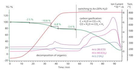
Time-dependent presentation of the release of CO,  $\rm CO_2$  and  $\rm H_2$  during carbon gasification in hydrous atmosphere (TGA curve in green, temperature curve in red)
