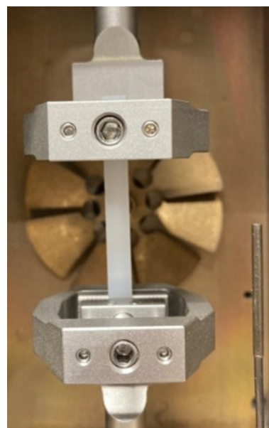
1 PE-HD in standard tension holder
