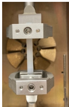
1 PE HD sample with dimensions of 55 x 5 x 2 mm in the employed sample holders
