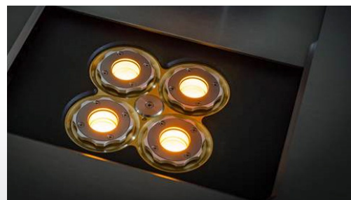
2 Four separate mini-tube furnaces of the LFA 467 HT HyperFlash®
