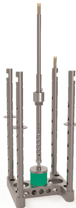
2 Position of the sample between the sample holder and pushrod for compression-mode measurements
