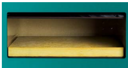
Various plate openings of the HFM 446 Lambda are possible when changing the specimen
