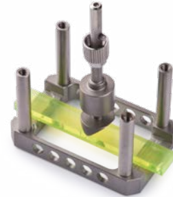
Sample holder for 3-point bending
