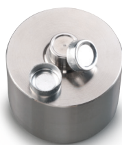
1 Photo of the SFI crucible and tool (left); cross-section of the SFI crucible (right)
