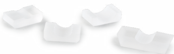
Sample-supporting kits made of fused silica
