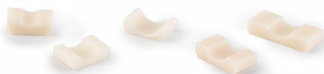
Sample-supporting kits made of alumina
