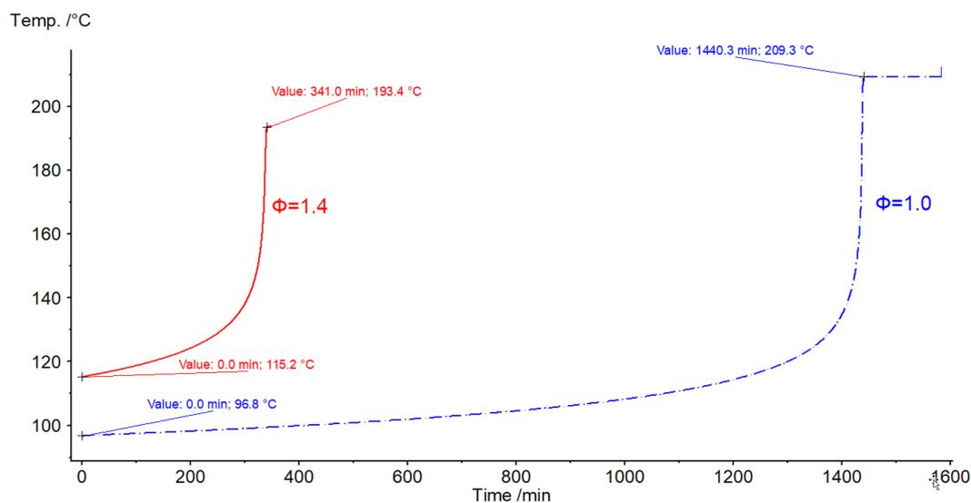
4 Non-linear TMR extrapolation for decomposition of 20-% DTBP in toluene. Red solid curve: experimental data for  $\phi=1.4$ . Blue dashed curve: simulated, non-linear extrapolation for  $\phi=1.0$  with  $T_{D24}=96.8^{\circ}\text{C}$ .
