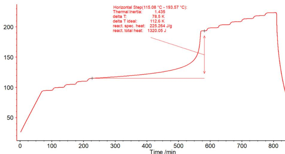
2 Decomposition of 20-% DTBP in toluene; measurement in Heat-Wait-Search mode (ARC 305 instrument).
