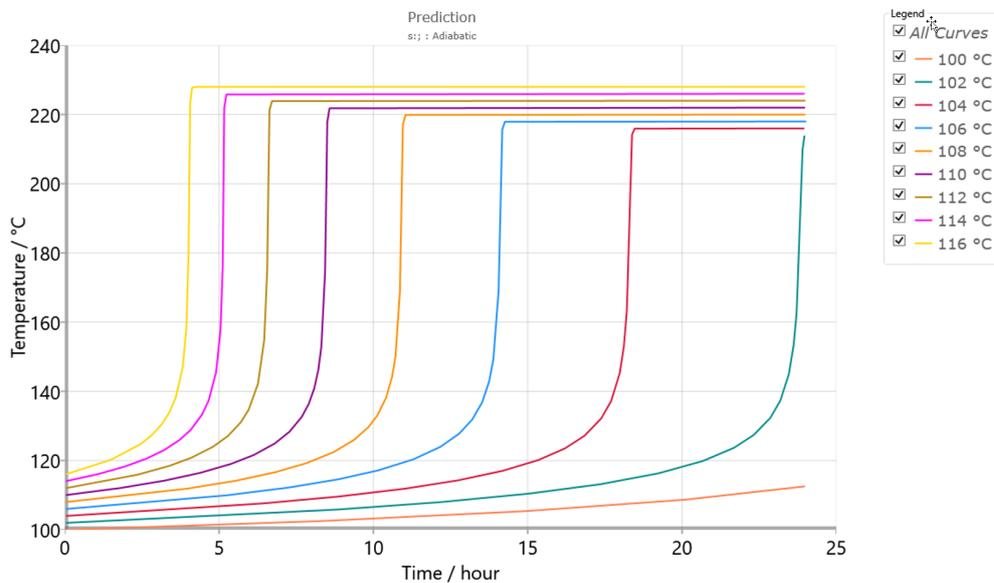
6 Simulation of the adiabatic self heating at different temperatures for  $\phi=1.0$ .
