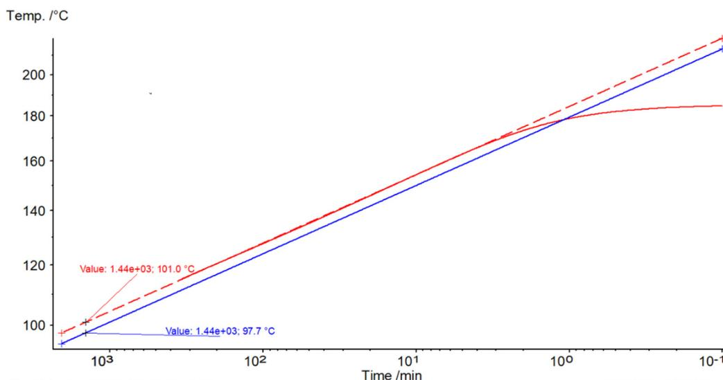
3 Linear TMR extrapolation for decomposition of 20% DTBP in toluene. Solid red curve: experimental data for  $\phi=1.4$  (figure 1); dashed red line: linear extrapolation for  $\phi=1.4$ ; blue line: simulated linear extrapolation for  $\phi=1.0$  with  $T_{D24}=97.7^\circ\text{C}$
