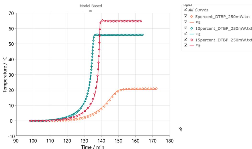
5 Temperature increase from ARC experiments (points) and simulations (solid lines) for DTBP in toluene for 5%, 10% and 15% solution under constant power of 250 mW. The one-step kinetic model of first order is found by model-based kinetic analysis.
