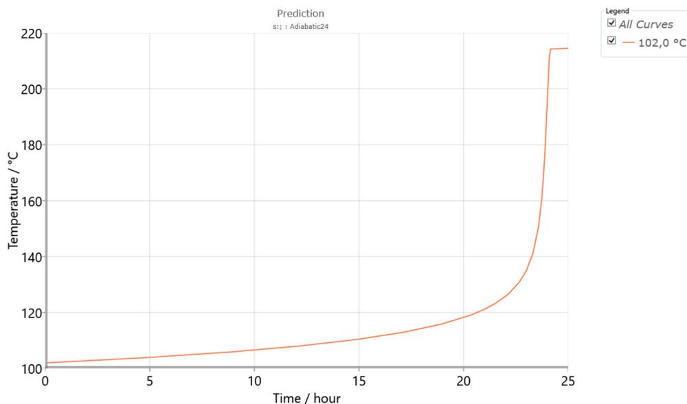
7 Calculation of  $T_{D24}$  for  $\phi=1.0$  and simulation of adiabatic self-heating at this temperature.
