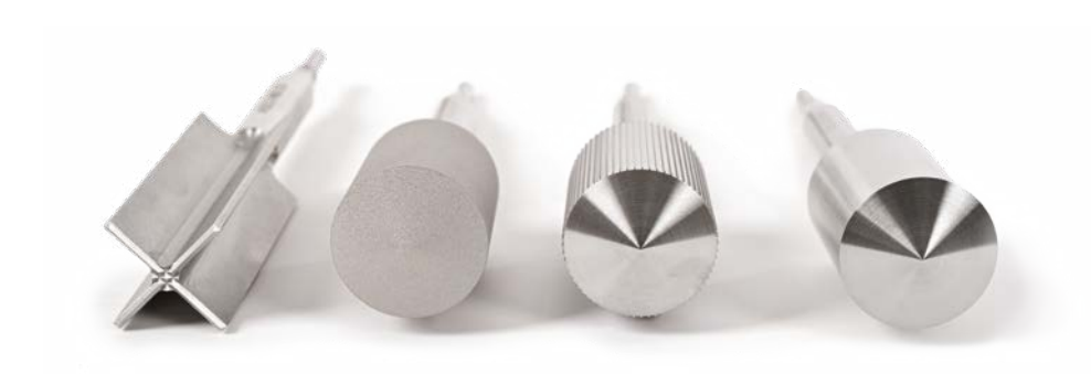
A 25mm diameter vane tool, roughened bob, splined bob and smooth bob
