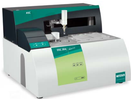
1 DSC 204 F1 Nevio with automatic sample changer.
