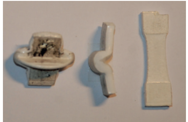
3 The contact force amplitude is essential to keep the test sample in planar shape (left: 0.5 N, center: 0.75 N; right: 1 N; \pm 0.5 N)
