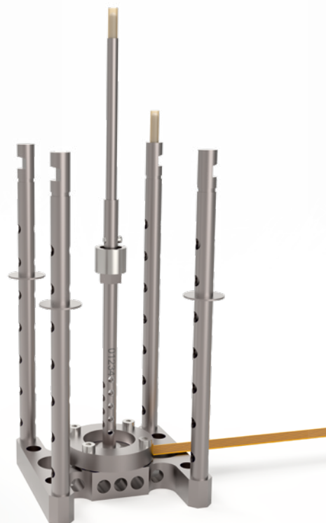
Sample holder for simultaneous DMA-DEA
