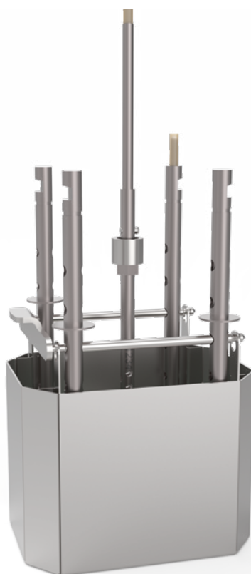
Liquid immersion accessory suitable for all available sample holders
