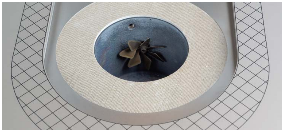
View into the DMA furnace with fan
