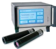
TRDA – Smoke Density Tester with light measurement system
