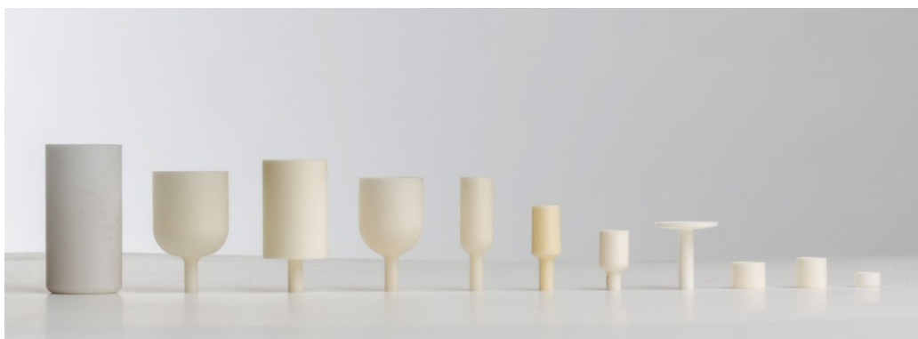
1 \text{Al}_2\text{O}_3 beakers or crucibles with volumes between 10 ml (left) and 85 µl (right).
