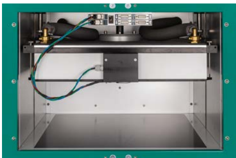
Open test chamber; 1-specimen measurement method
