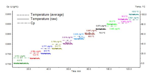
1 Results of the specific heat capacity on sapphire during quasi-isothermal measurement
