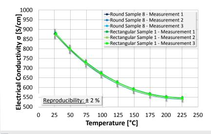
7 Three measurements each of the electrical conductivity of a round and rod sample of the BiSeTe material
