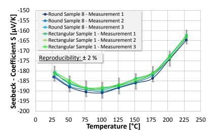
6 Three measurements each of the Seebeck coefficient of a round and rod sample of the BiSeTe material
