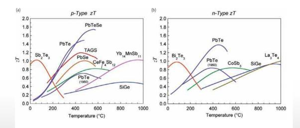
3 Approximate Figure of Merit (ZT) for various p-type and n-type thermoelectric materials Source: G. Jeffrey Snyder, California Institute of Technology http://thermoelectrics.caltech.edu. Reproduced with permission.
