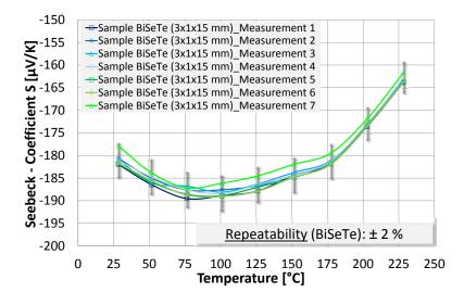
4 Multiple measurement of the Seebeck coefficient of a BiSeTe sample
