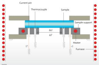
2 Schematic diagram of the SBA 458 Nemesis®
