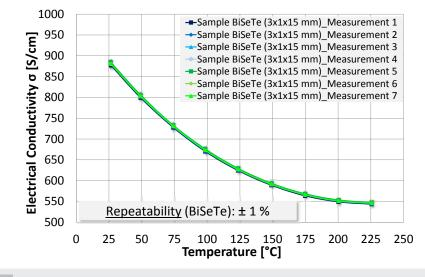
5 Multiple measurement of the electrical conductivity of a BiSeTe sample
