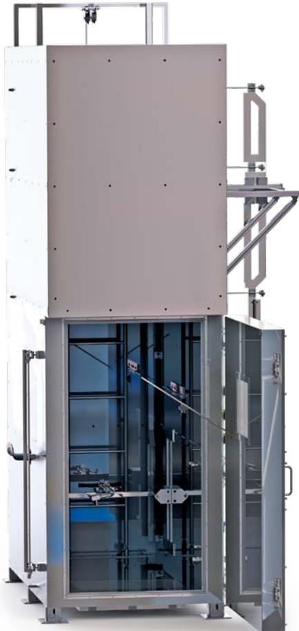
Test chamber with burner and sample holder (ladder)
