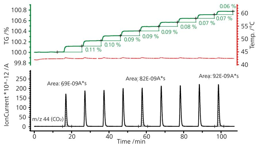
Isothermal treatment of CaO (177.8 mg) on a Pt grid sample carrier at 43°C in a dry argon atmosphere with pulses of 250 µl of CO<sub>2</sub>
