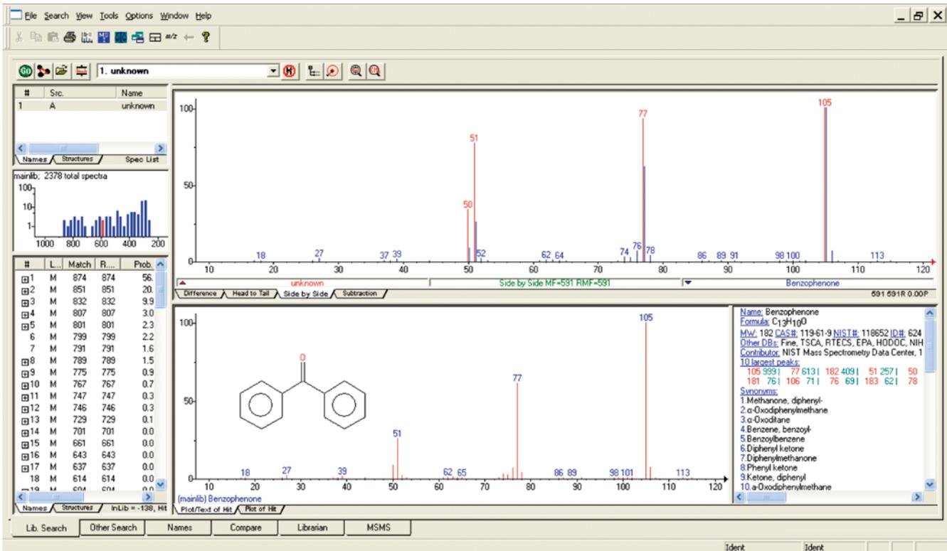
Direct export of the MS results at 166°C into the NIST database for identification of the evolved gases
