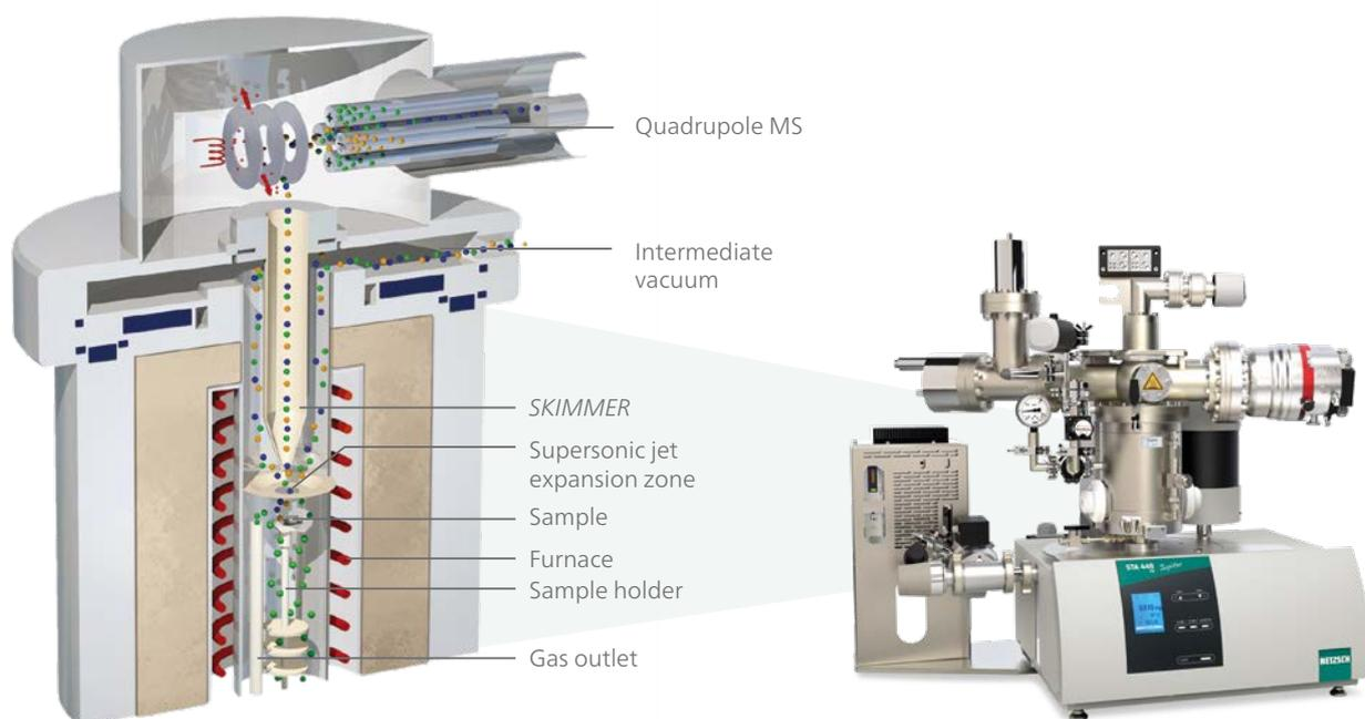
*Shortest possible coupling solution via special supersonic jet gas transfer*
