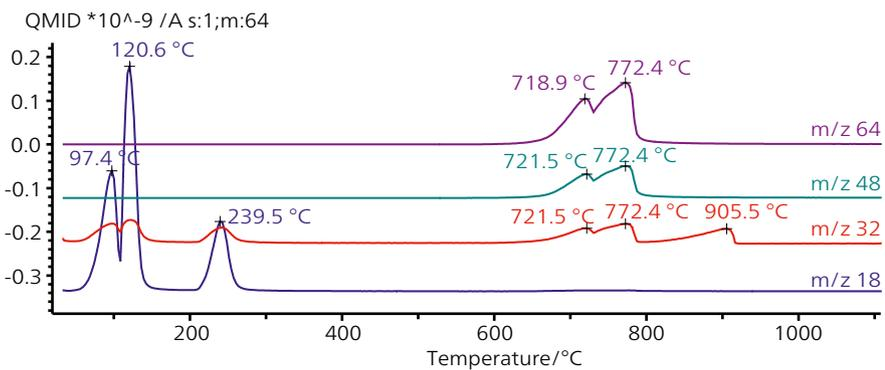
Thermogram of blue vitriol in combination with the ion current curves of m/z 18, 32, 48 and 64
