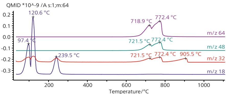
Thermogram of blue vitriol in combination with the ion current curves of m/z 18, 32, 48 and 64
