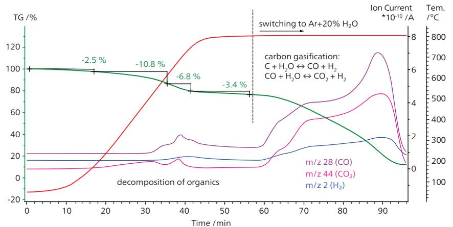
Time-dependent presentation of the release of CO, CO<sub>2</sub> and H<sub>2</sub> during carbon gasification in hydrous atmosphere (TGA curve in green, temperature curve in red)
