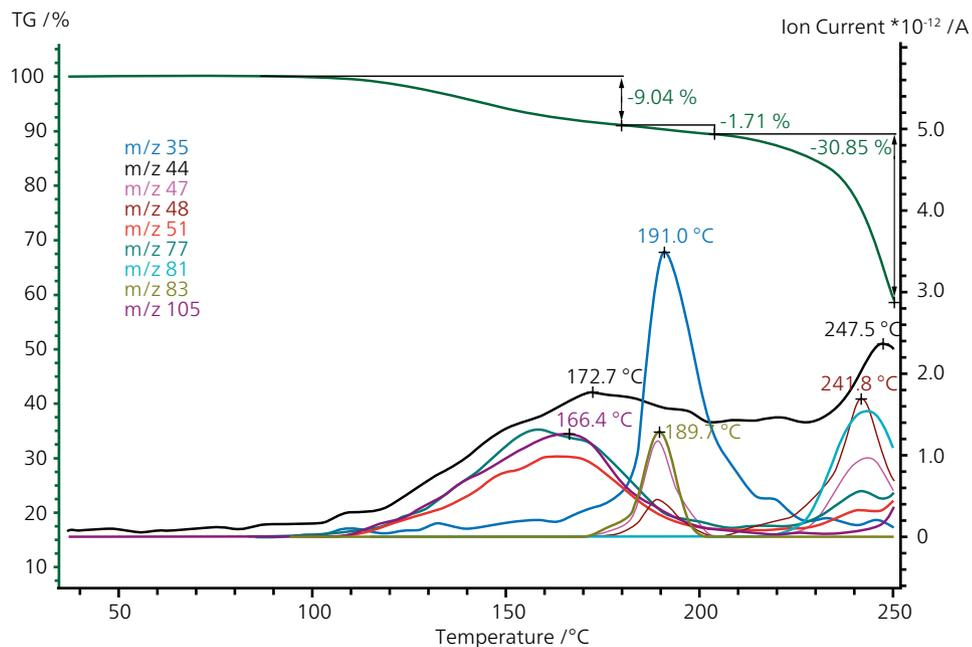
Correlation of the mass loss steps and the detected gases. m/z 35 can most likely assigned to HCl.
