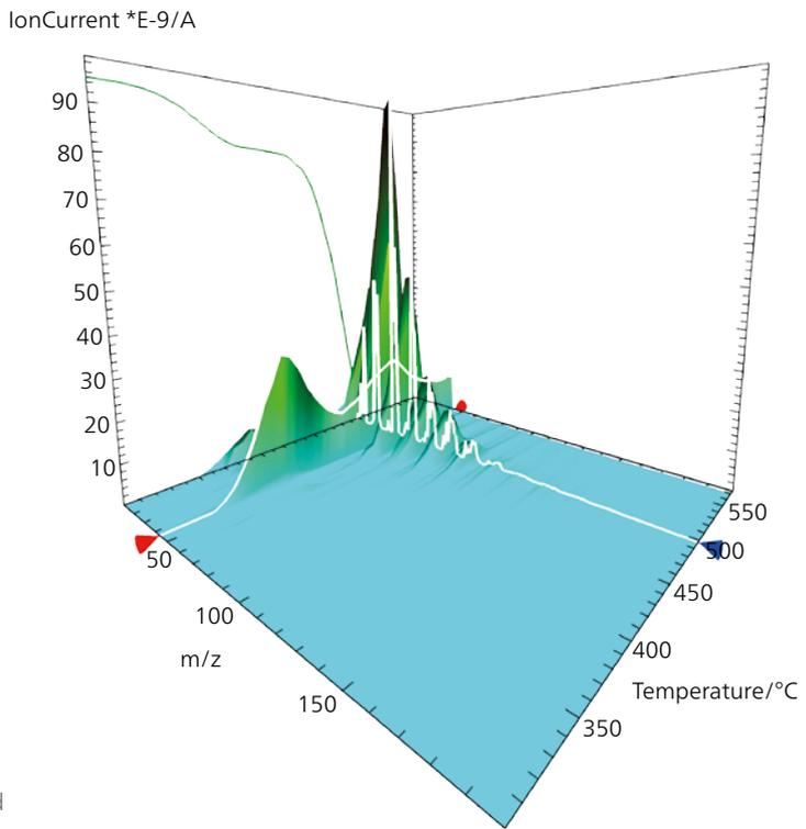
The 3D plot of temperature, m/z ratio and ion current depicts all MS data within one graph. It enables visualization of the relationship between mass loss and the signal increase in the individual m/z numbers.
