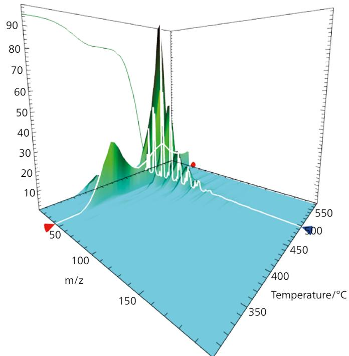
The 3D plot of temperature, m/z ratio and ion current depicts all MS data within one graph. It enables visualization of the relationship between mass loss and the signal increase in the individual m/z numbers.
