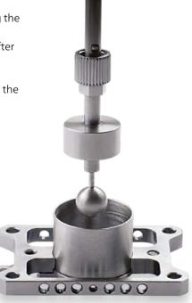
The ball-shaped pushrod is immersed in the sample during measurements with sample holder set DMA2420CA55.010-00.
