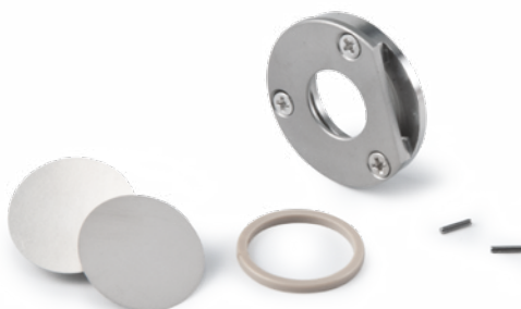
Sample holder for liquids “PEEK”, order no. 6.256.4-92.7.00
