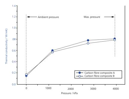
LFA 457 *Microflash* <sup>o</sup> measurements on two carbon fibers (2 mm thick) between ambient and 4 MPa in air at room temperature.
