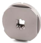
Standard sample holder, 8.0 mm x 8.0 mm, order no. LFA46700A90.044-00
