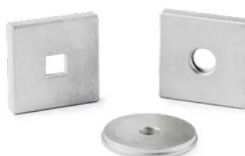
Sample holders and mask for round and square samples – 8.0 mm
