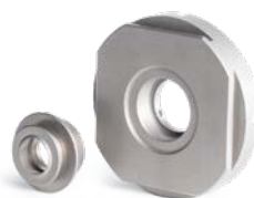
Sample holder for thick samples, order no. LFA46700A90.086-00
