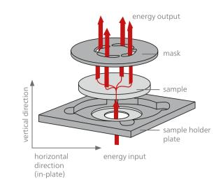
Heat flow directions using the in-plane sample holder. The special set-up of the in-plane sample holder eliminates the typical measurement limitations caused by the minimum sample thickness.
