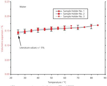
LFA measurements on water between RT and 85°C (sample thickness 1.5 mm).
