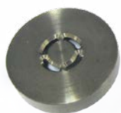
Sample holder for in-plane measurements, order no. 6.257.1-91.2.00
