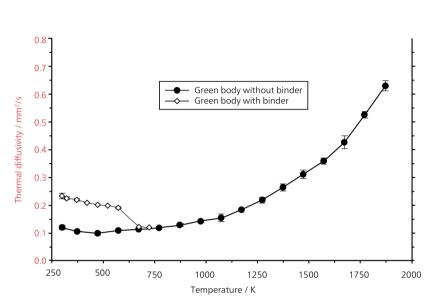
Thermal diffusivity of zirconium oxide green bodies measured in the LFA 427
