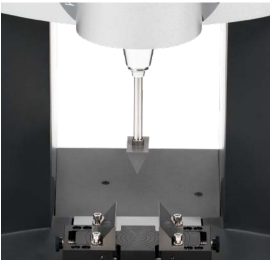
Kinexus ultra+ equipped with the universal container holder and the texture analysis 3 point bend kit (KNX2292)
