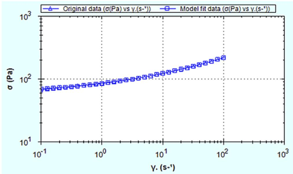
2 Shear stress-shear rate data for the Carbopol-based hair gel with Herschel-Bulkley model fit
