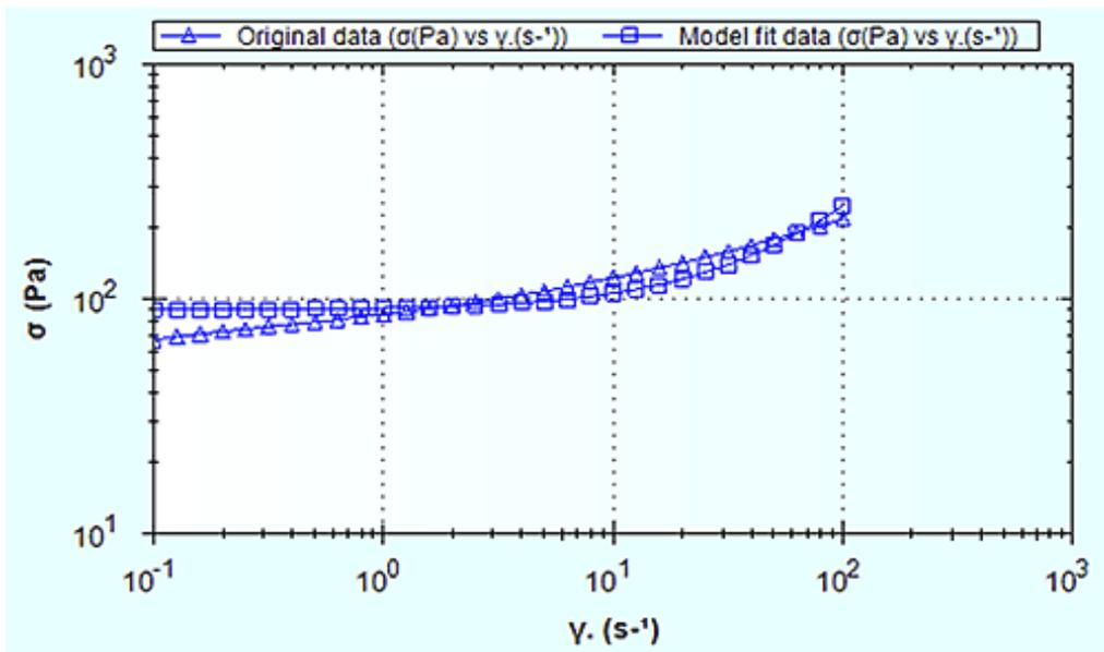
3 Shear stress-shear rate data for the Carbopol-based hair gel with Bingham model fit
