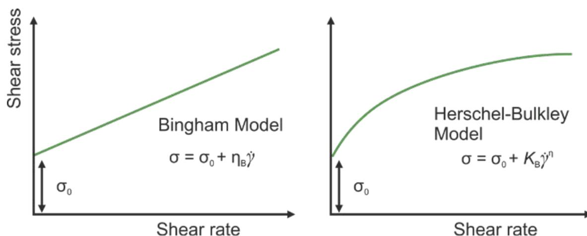
1 Illustration of Bingham and Herschel-Bulkley model fits using linear scaling
