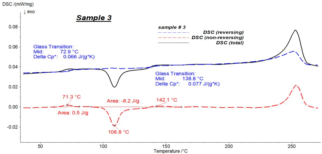
**6** Results of modulated DSC measurements on PET/PC3 during the first heating
