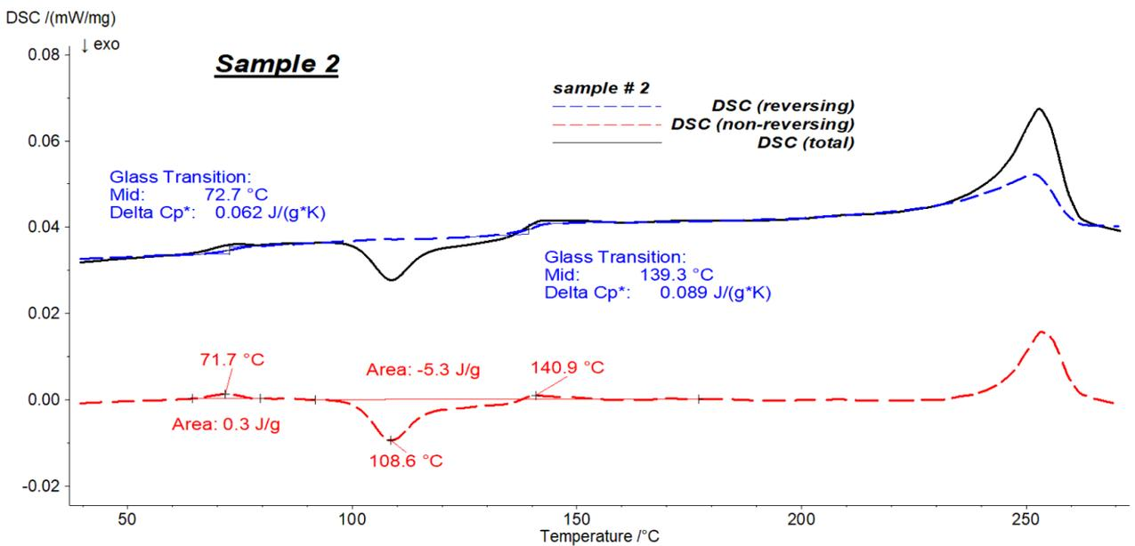
5 Results of modulated DSC measurements on PET/PC2 during the first heating
