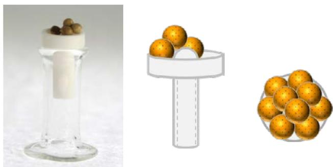
Fig. 6a. Original and 6b+c. Illustrated application of the trimmed  $Al_2O_3$  crucible for the A- $CaCl_2$  composite granules (yellow)
