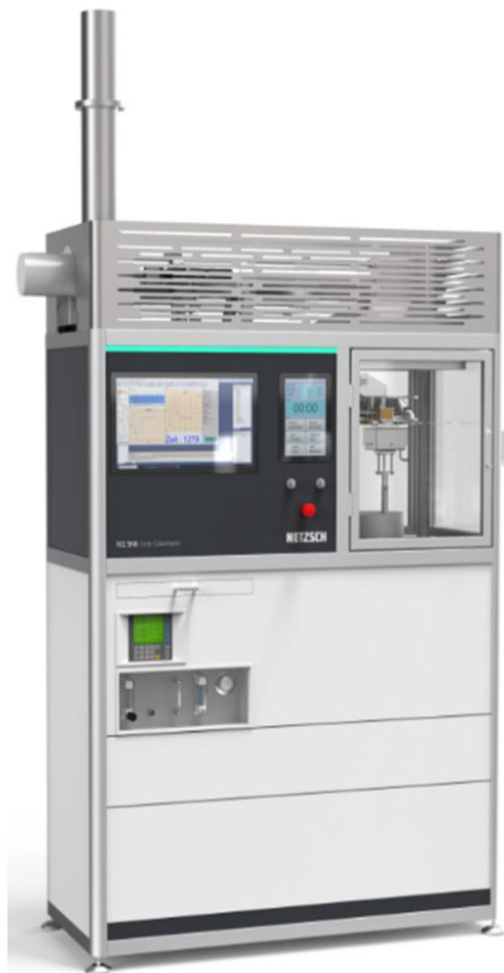
1 Cone Calorimeter TCC 918
