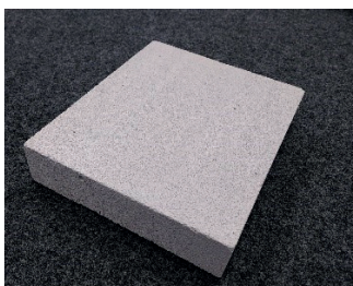
3 Porous concrete – Specimen 1 (left); porous structure in a breaking edge (right)
