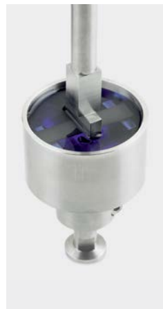
3 – Point bending with immersion bath
