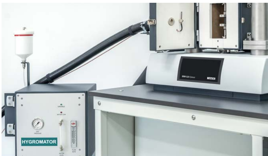
Humidity generator connected to the standard furnace
