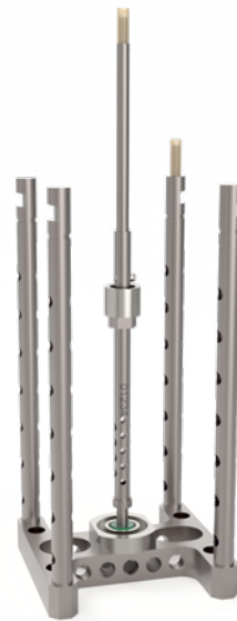
Sample holder for measurements on pasty samples in compression with insert
