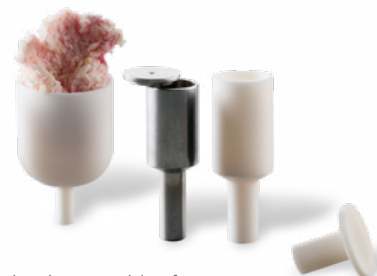
Large beaker crucibles for high-volume TGA tests
