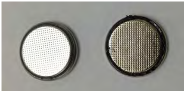
6 LiR2032 coin cell before and after DSC scan to 300°C
