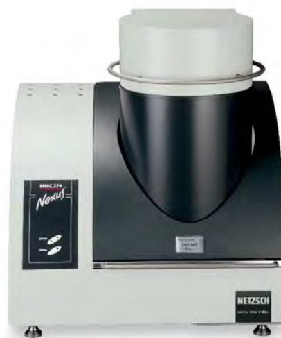
1 The high-temperature coin cell module on MMC 274 Nexus ®
