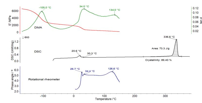
6 DSC, DMA and rheometer measurements. Black: DSC. Red: Storage modulus  $E'$  (DMA). Green: Loss factor  $\tan \delta$  (DMA). Blue: Phase angle  $\delta$  (rotational rheometer).
