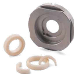
Sample holder for fibrous samples, order no. 6.256.1-93.3.00
