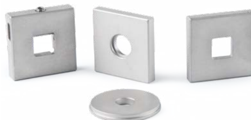
Sample holders and mask for round, square and laminated samples – 12.7 mm
