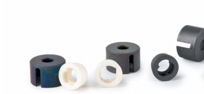
Centering cones and caps for round and square samples (diam. of 10 mm); centering cones made of \text{Al}_2\text{O}_3 (white) and graphite (grey); caps made of SSiC and graphite.
