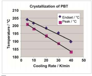
**3** Correlations of the endset and peak temperatures of PBT, measured at different cooling rates (see figure 2)
