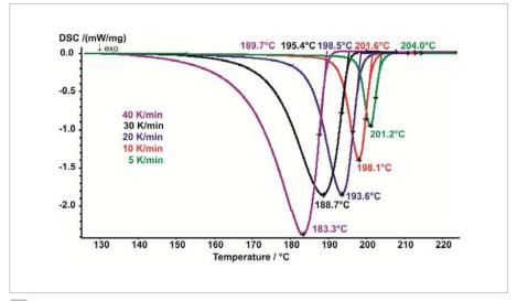
2 Influence of the cooling rate on the crystallization behavior of PBT, measured with the DSC 204 F1 Phoenix®
