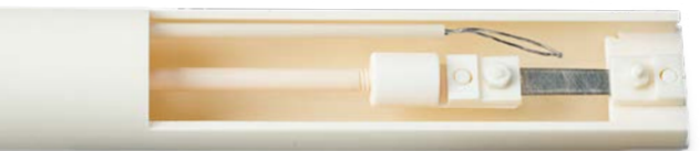
Tension sample holder kit made of alumina
