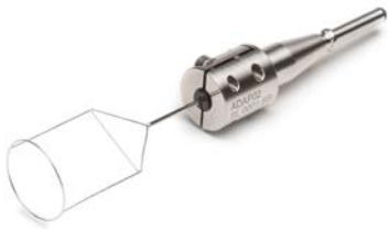
Du Nouy Ring (KNX4041) with Custom Geometry Adapter (KNX2174)
