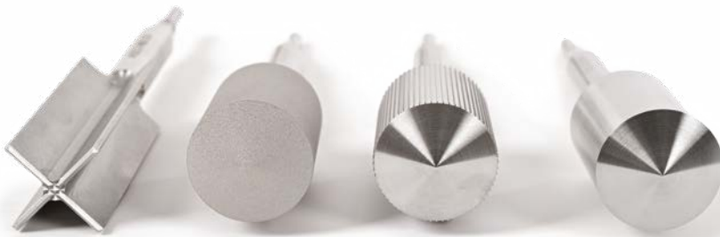
A 25mm diameter vane tool, roughened bob, splined bob and smooth bob
