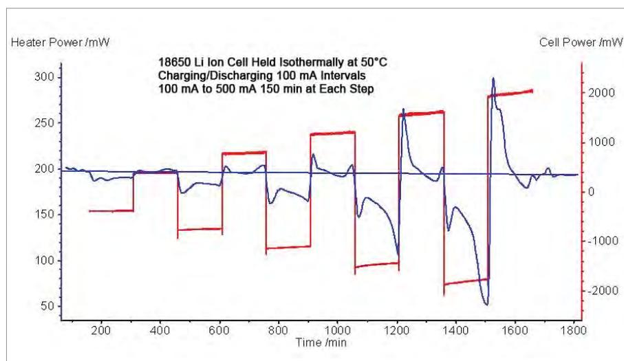
5 Cell heater power and cell current versus time for an isothermal 18650 battery cycling test at 50°C with increasing current
