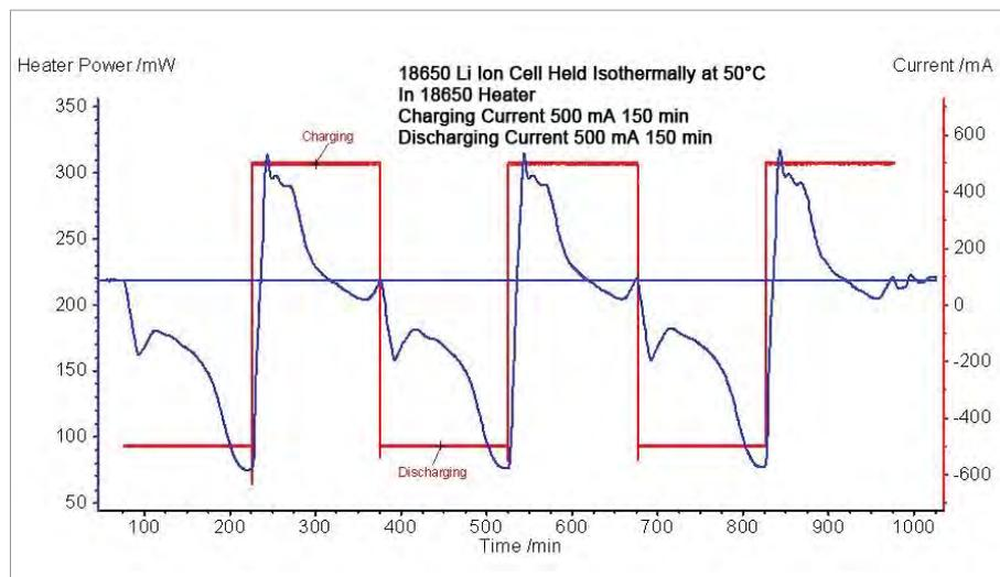
4 Cell heater power and cell current versus time for an isothermal 18650 battery cycling test at 60°C
