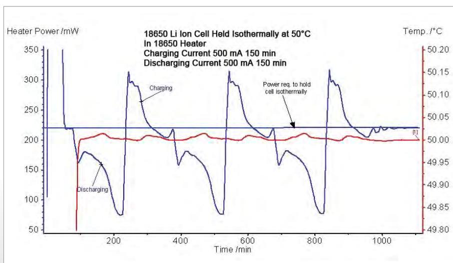
3 Cell heater power and cell temperature versus time for an isothermal 18650 battery cycling test at 50°C
