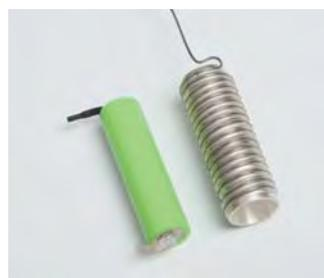
2 18650 cell and its *VariPhi*<sup>TM</sup> sensor
