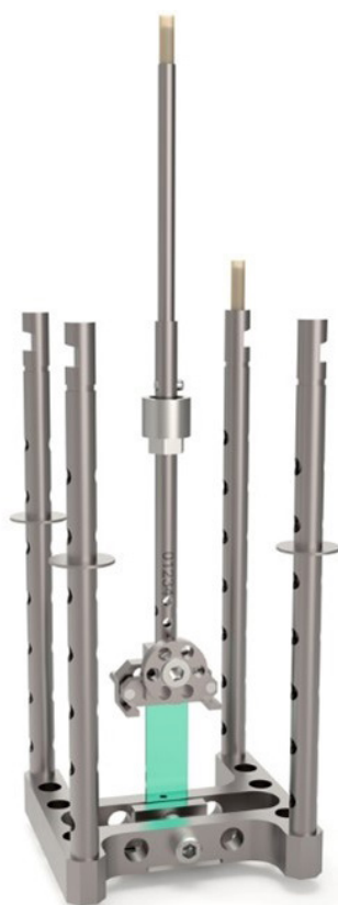
1 Schematic of a thin rectangular sample placed within the steel tension sample holder.
