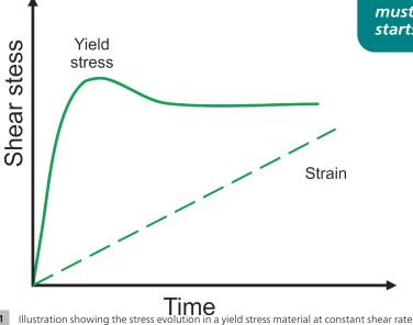
Yield stress is defined as the stress that must be applied to the sample before it starts to flow.
