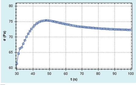
2 Stress ( $\sigma$ ) versus time curve for a body lotion sample run at a constant shear rate of 0.01 s<sup>-1</sup>
