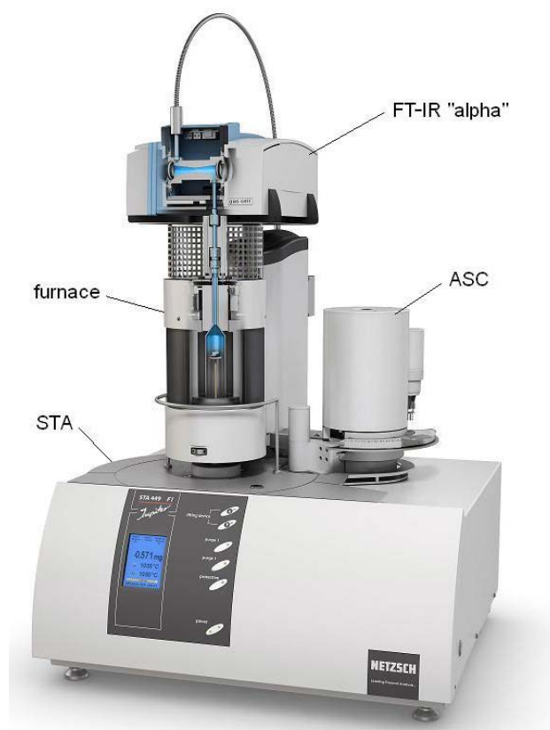
1 NETZSCH Perseus STA 449: The Bruker type "Alpha" FT-IR spectrometer coupled directly to a simultaneous thermal analyzer STA 449 Jupiter ® equipped with an optional automatic sample changer (ASC). The sample space of the furnace, the heated coupling interface as well as the gas cell of the FT-IR spectrometer are shown partially transparent in order to display the path of the evolved gases [1].
