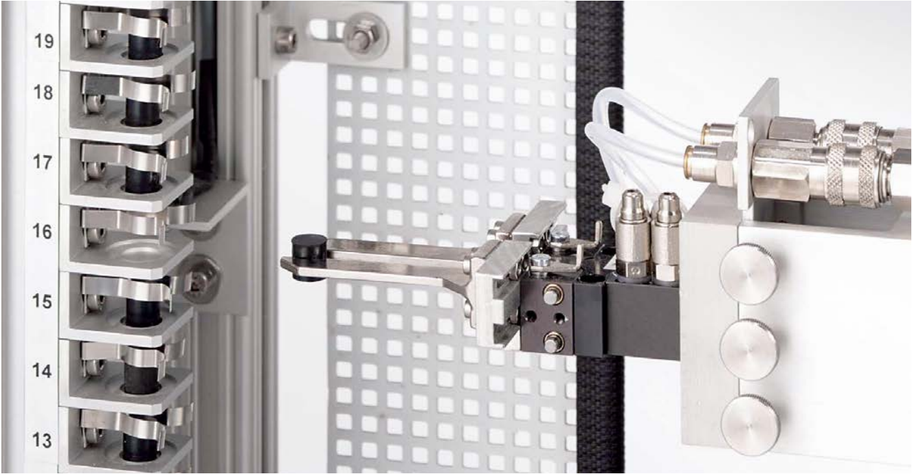
Autosampler (ASC) for compression mode; only the specimen is changed out
