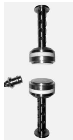
Combined DEA and DMTA sample holder for small samples
