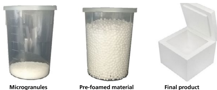
Fig. 1. Blowing-agent-loaded polystyrene microgranules, pre-foamed beads and the final EPS product
