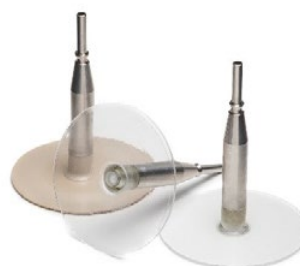
Fig. 3. Alternative material upper plate geometries: PEEK and acrylic
