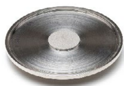
Fig. 2. Lower pedestal plate to match a 20-mm upper geometry. Roughened surface finish.
