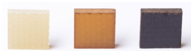
Fig. 3. Typical color change as a sign of beginning degradation: left before measurement, in the middle after being measured at 260°C and right hand side at 300°C.
