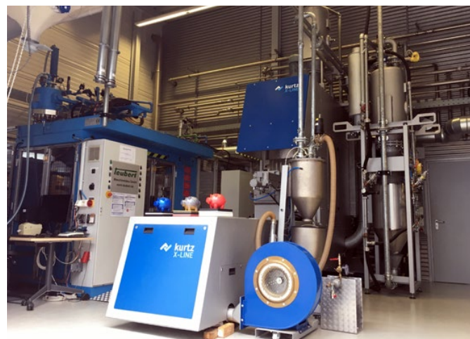
Fig. 2. Steam-chest molding machine (on the left) and pre-foaming unit (on the right) for production of the EPS parts
