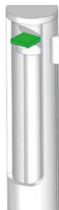
1 Fixture set for 3-point bending made of fused silica, bending length: 5 mm.
