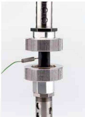
3 Sample arrangement with needle thermocouple
