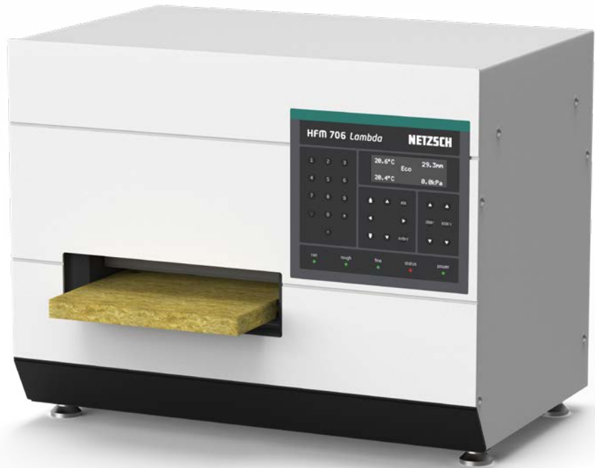
Inserting the reference material; various reference materials can be used
